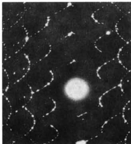
Fig. 4. Hyperbolic loci of diffraction groups from a single \text{MoS}_2 crystal rotated about an axis normal to beam (its projection is vertical in Fig. 4).
