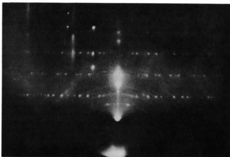
Fig. 1. Layer-line pattern from silver nitrate, showing high perfection of orientation sometimes obtained in deposits formed on substrates which are atomically highly smooth, in this case smooth {111} faces of silver crystals on a muscovite mica cleavage face.
